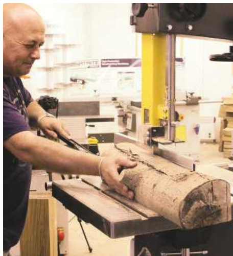
Pic.4 Now you have two square faces bearing on the table and the fence; the King squint is optional but strikes fear into timber
